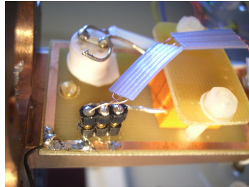
Cold FET board HV contact
