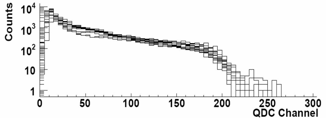
Calibrated QDC pulse height spectra
