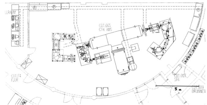
Figure 1: Jena AMS system: recombinator:  $4 \times 45^\circ$  magnets, Tandatron model 4130: terminal voltage 3 MV, high energy mass spectrometer:  $110^\circ$  analyzing magnet,  $33^\circ$  electrostatic analyzer,  $90^\circ$  magnet, two anode gas ionization counter[6, 7, 8]. Shown is also the new MICADAS AMS system [3].
