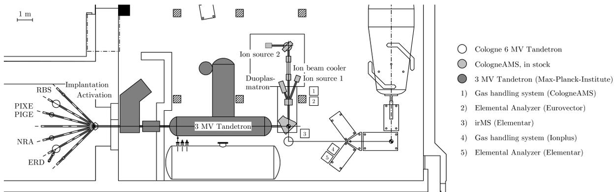
Figure 2: One possible opportunity for the set-up of the new 3 MV Tandatron accelerator in the second basement of the accelerator building (Institute for Nuclear Physics, University of Cologne). Shown are the new components from the MPI (dark gray), the available components of the IKP (light gray) and ion beam lines for future applications; e.g. RBS, PIXE, PIGE, NRA and ERD.
