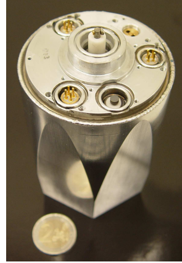
Figure 2.2: Picture of a 12-fold segmented encapsulated MINIBALL crystal.
