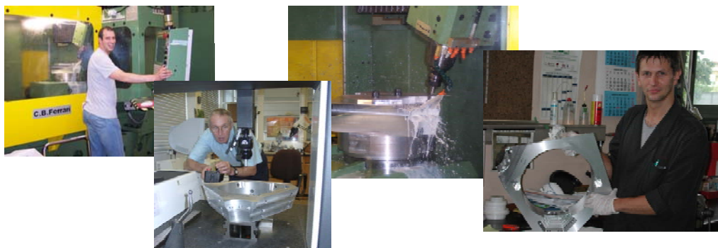
Figure 16.8 Images of the flanges being machined and inspected
