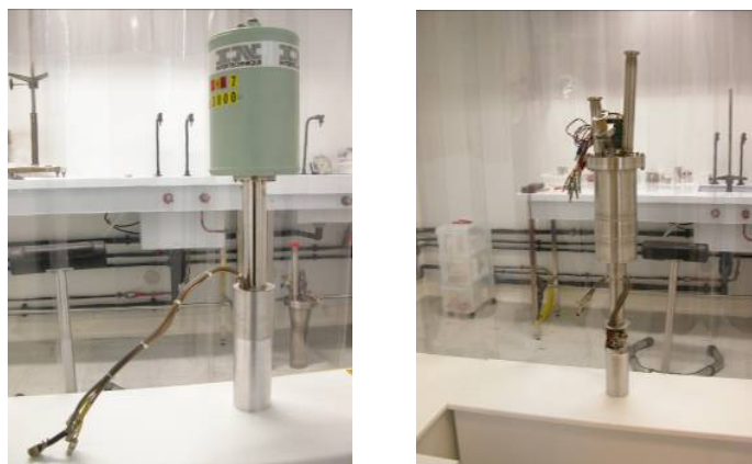
Figure 22.9: Detector used for He Loop. Left : Eurisys cryostat. Right : IPNO cryostat.
