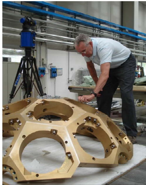
Figure 16.10 Flanges being positioned using the laser tracker
