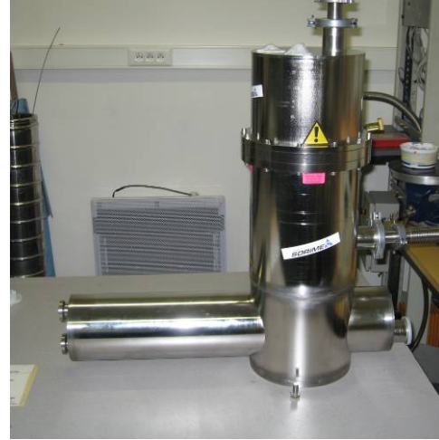
Figure 22.10: Drawing (left) and photograph (right) of the thermal shunt.
