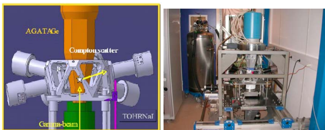
Fig. 7.2. Drawing (left) and photo (right) of the Orsay scanning system: 6 NaI modules of TOHR and mechanical support, the AGATA detector and the collimated intense ^{137}\text{Cs} source.
