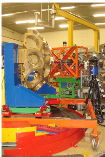
Figure 16.15 Using the laser tracker to position the generic support structure
