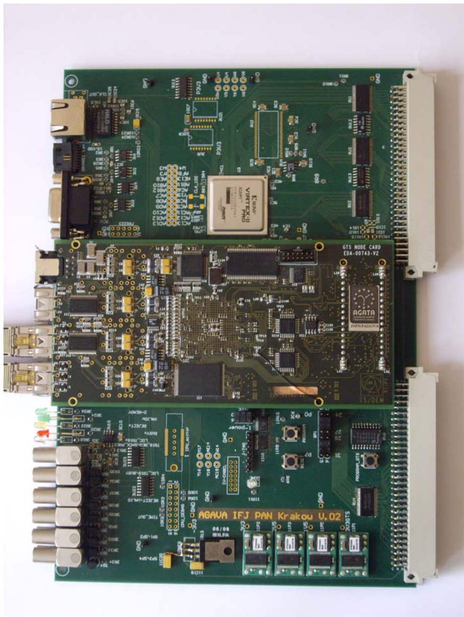
Fig.14.3 Top View of the AGAVA board with GTS mezzanine card.
