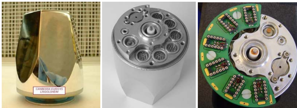
Fig. 5.3. Pictures of the AGATA unsegmented crystals. (left) encapsulated crystal, (centre) encapsulated crystal with PCB (right).
