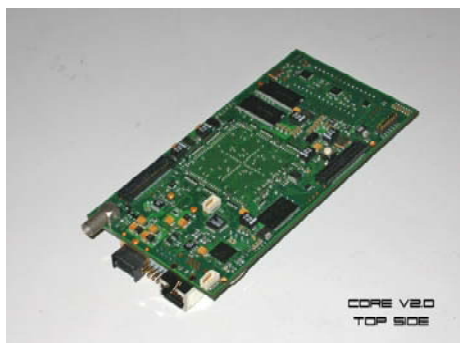
Carrier card equipped with 4 mezzanines
