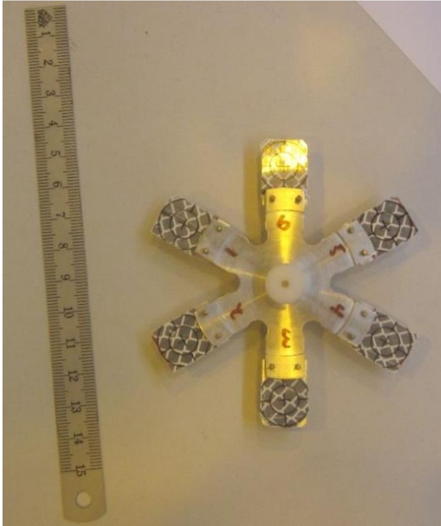
Figure 4: The Leica retro-reflective targets mounted on the Miniball target wheel
