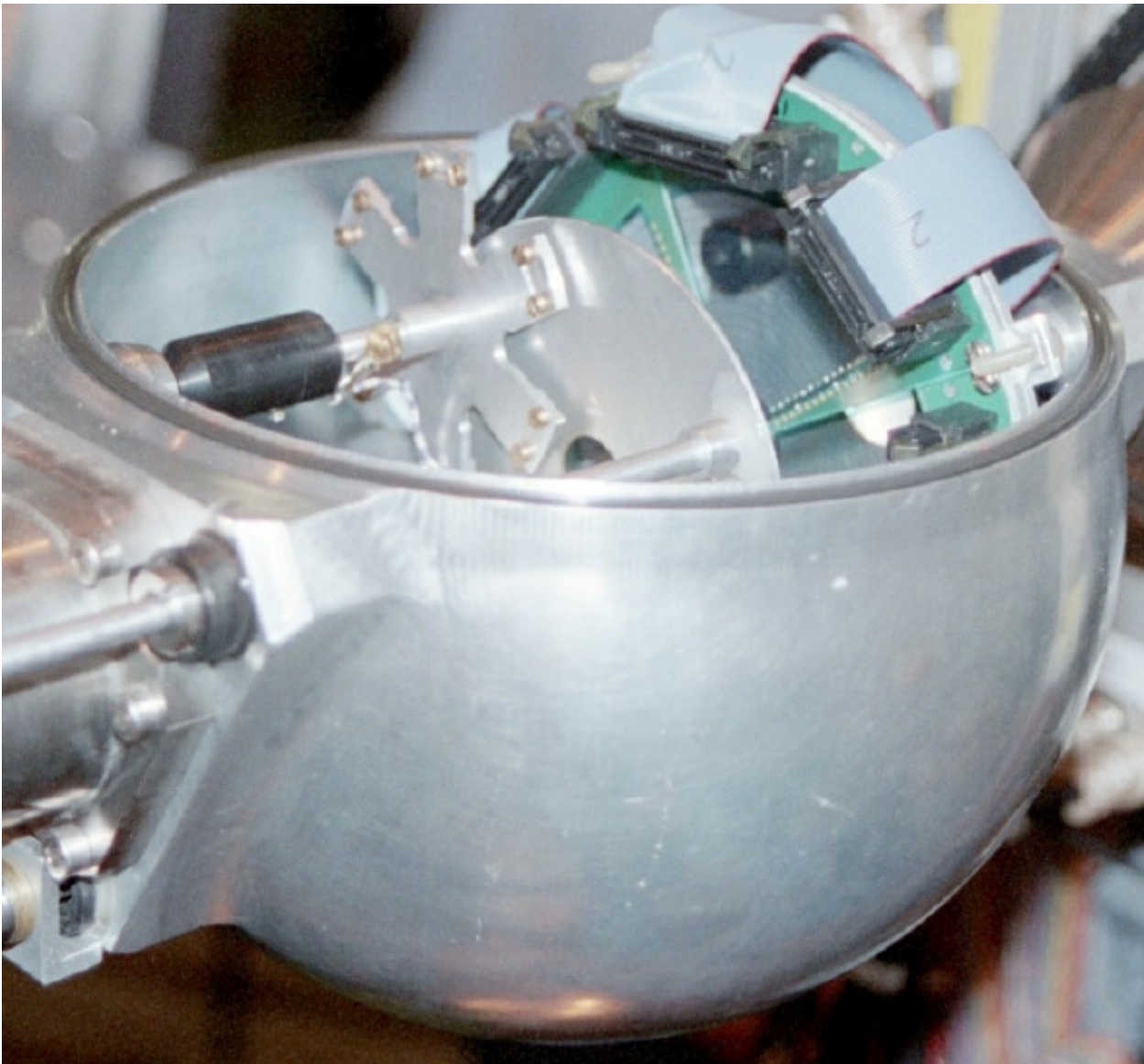
Figure 9: The CD mounted in the target chamber. You can see the target wheel and the CD protection plate (which is no longer used) with the CD behind it.
