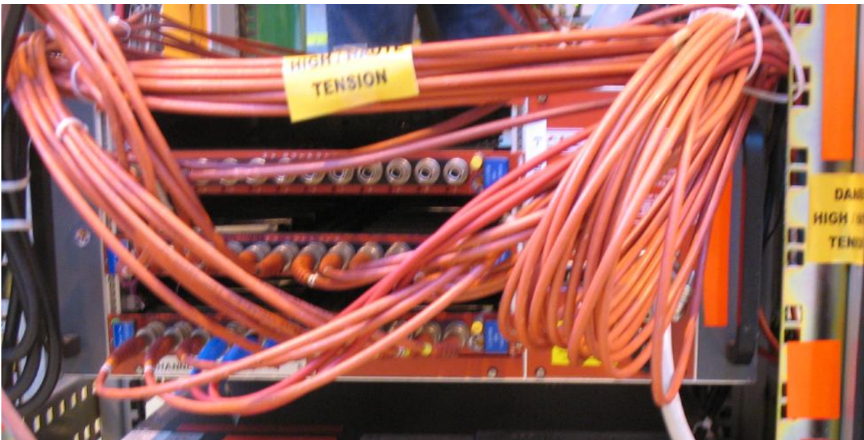
Figure 51: R5 rear: HV connectors. Note that the bottom card is the first one with channels 0 to 11 and we only use one channel of the third card for the beam-dump detector
