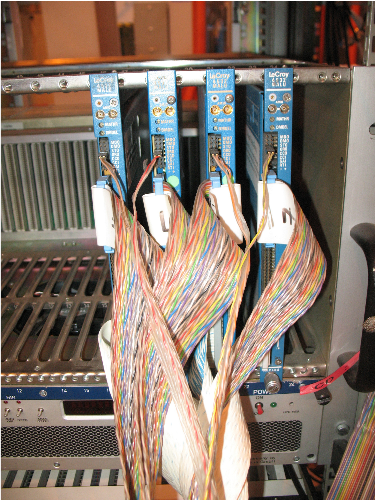
Figure 32: R1.C2: The cabling of MALUs - four multicoloured flat cables (one from each quadrant - the other ends are split in pairs, so they go to 8 RAL109s) come from the RAL109s in R2.C2 (i.e. the front rings) to the inputs. Four blue and white flat cables go from the outputs of the MALU to the TDCs. The ORO output of each MALU goes to the ECL→NIM converter (R1.C3.S23).
