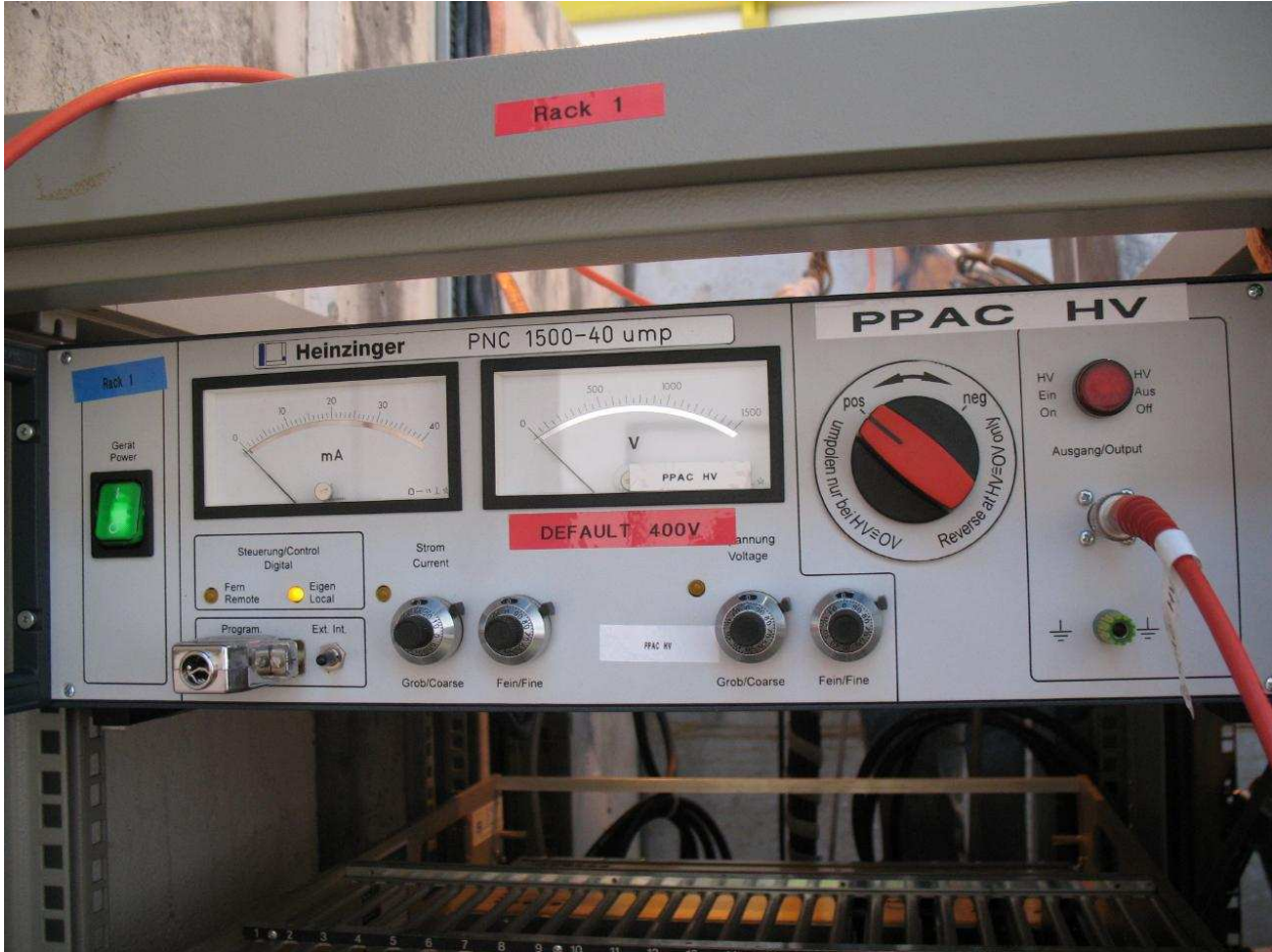
Figure 19: R1.C1: PPAC power supply. We normally use about +400 Volts
