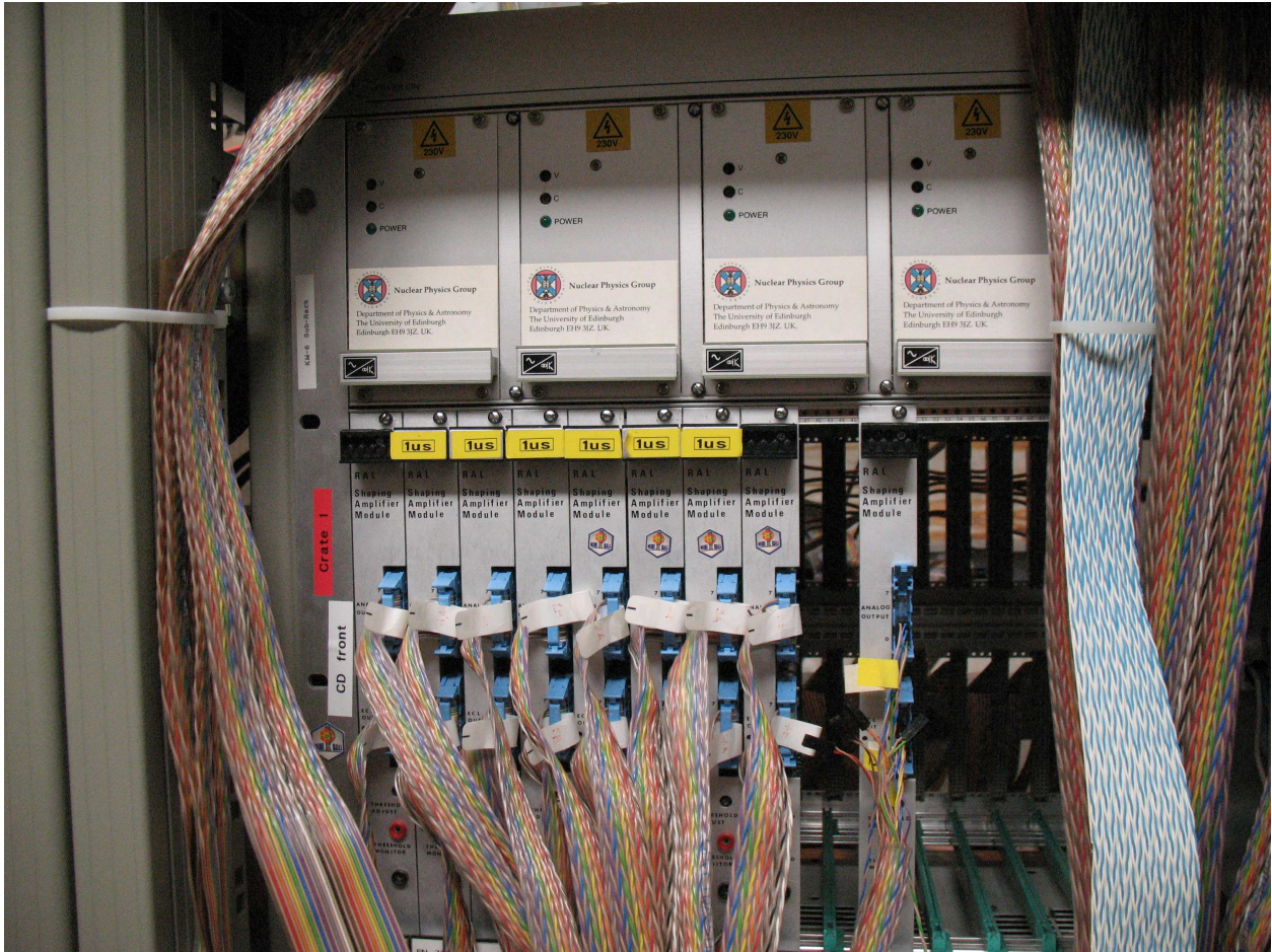
Figure 28: R2.C1: The RAL109s for the front rings. The upper connections are for the energy and they are joined up in pairs and sent to the ADC. The lower connections are for the timing and they go to the MALU in R1.C2 and from there to the TDCs in R3.C1.
