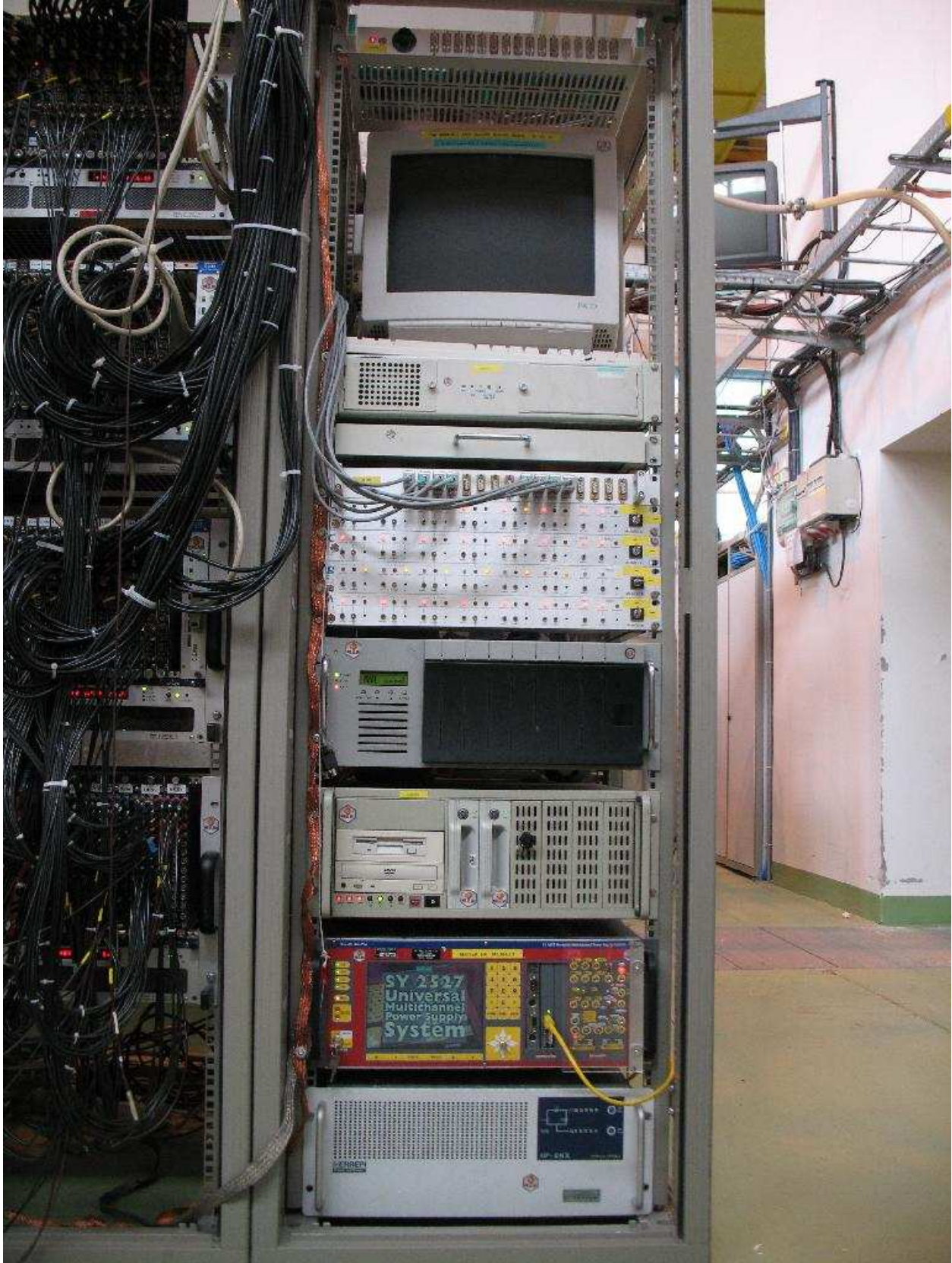
Figure 54: R5 bottom: filling system computer with monitor and keyboard, new PT100 box and four manifold controller boxes, raid array, DAQ computer, CAEN HV power supply and UPS. The old PT100 box is above the monitor.
