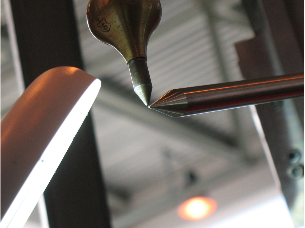
Figure 15: Alignment: the tip of the brass “plumb” bob was aligned to the target position. The tip of the metal spike mounted in a detector ring was then aligned to this.
