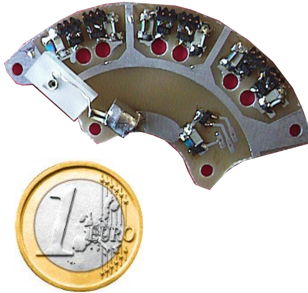
Figure 12: The cold part of the preamplifier, with a Euro coin for size comparison. This is out of date.
