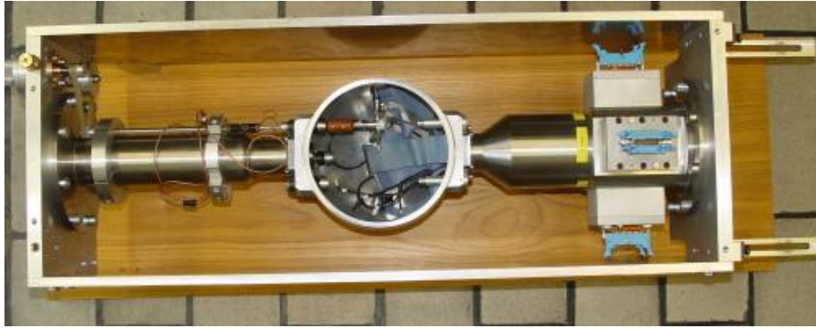
Figure 1: View of the target chamber from above. In this picture, the beam goes from left to right. Inside the target chamber the CD is not mounted, but you can see its cables and the feedthroughs. The PPAC flange is also not mounted. Note, however, that from 2007, the PPAC was no longer mounted in the position indicated, but further down stream on an actuator.
