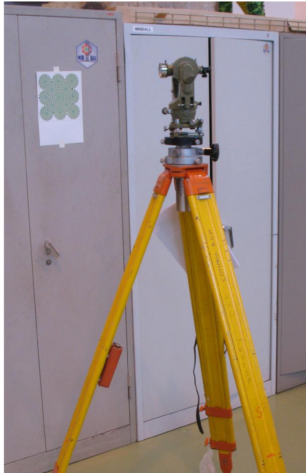
Figure 1: The Wild T1A theodolite on its tripod.
