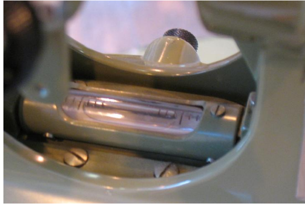
Figure 7: The tubular spirit level with the bubble in the middle. Note this is much more sensitive than the two dimensional one, but you have to rotate about the vertical axis to check the whole plane, not just a line.
