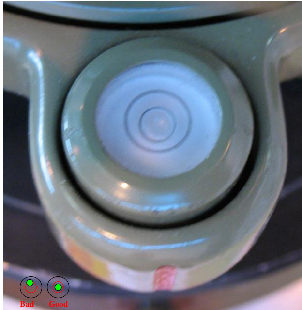
Figure 5: The 2-d spirit level with the bubble in the middle indicating the base is more or less horizontal.
